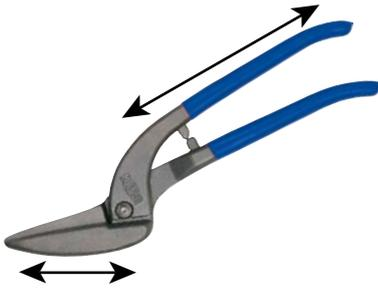
In normal metal snips, edges and handle are traditionally forged into one unit. The force required for cutting is determined by the ratio of edge length to the handle length.
