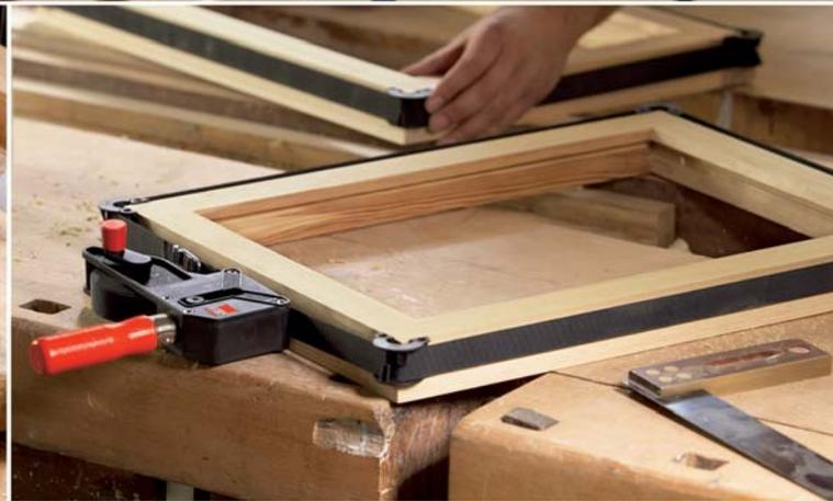
**For even clamping on both sides without warping or skewing of the workpiece**
