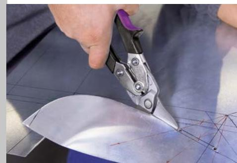
\* Snips can be stressed for up to 3 x 0.6 mm (1.8 mm) for a short period of time for cutting the seams.
