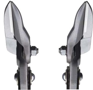
Right cutting snips are sharpened and designed so that they can cut right radii (i. e. a curve **from left to right**) easily. Left cutting snips are the best for radius cuts **from right to left**.
