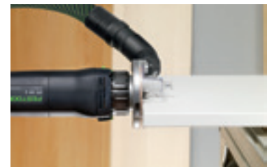
Rounding plastic or solid wood veneer.
